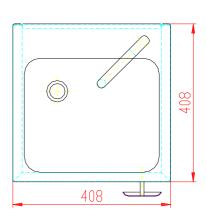
The washbasin is made of stainless steel and knee operated. The operation system is placed in right bottom of the front plate. To the water pipes is the washbasin connected with two angle valves (hot and cold water) that allow water temperature setting. The outlet drains the wastewater. The stainless steel washbasin with its construction and design answers to the high demands on cleanness and hygiene in food industry.
